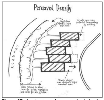
Figure 25: Design to reduce perceived density
