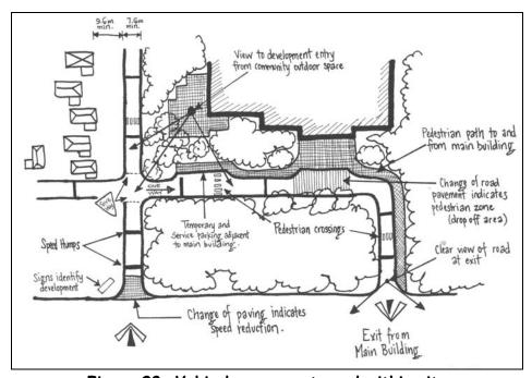
Figure 28: Vehicular access to and within site
