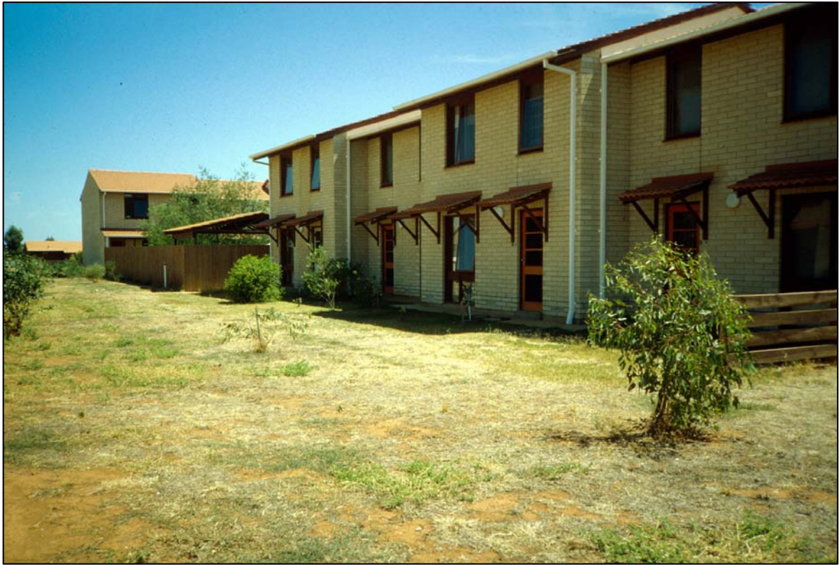
Figure 14: No differentiation of private yards from shared open space compromises dwelling privacy
